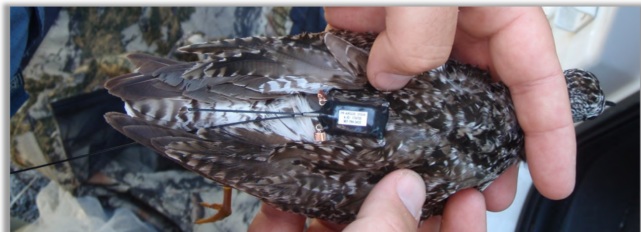
GPS Pinpoint Tag on a Lesser Yellowlegs near Yellowknife, NT. (Photo by Ross Wood)
