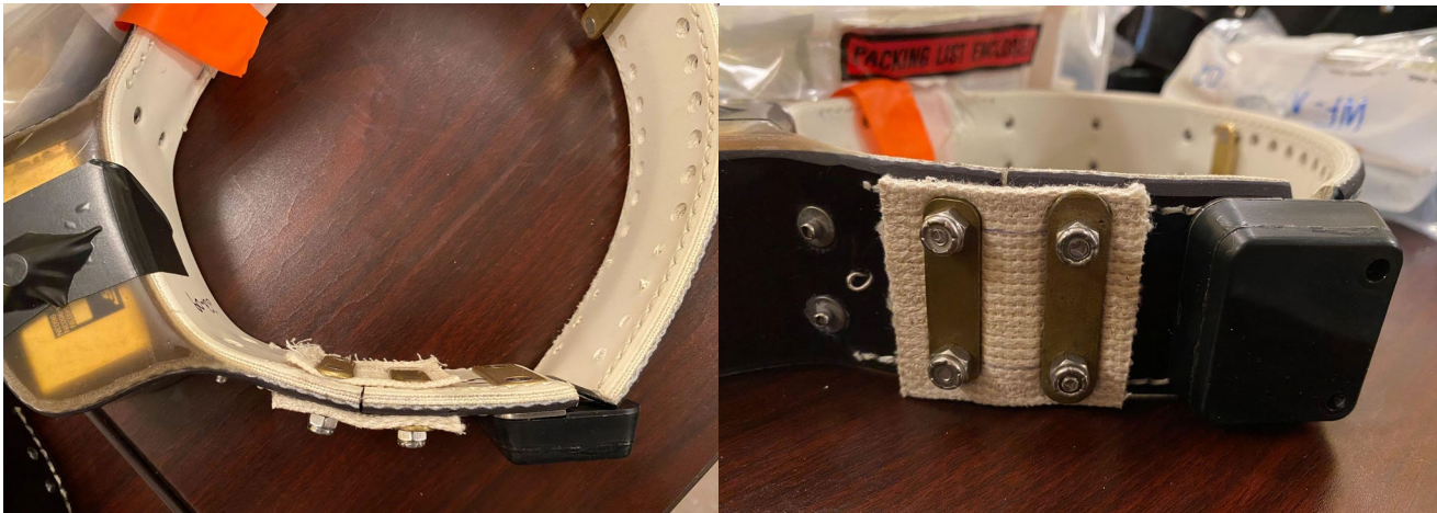
Figure 3. Wolves were fitted with Telonics (Model TGW-4577-4) GPS collars that were designed to lay flush against the neck and contain both a cotton breakaway and a timed-release mechanism (black box). Photos taken by Abbey Wilson, GNWT-ECC.
