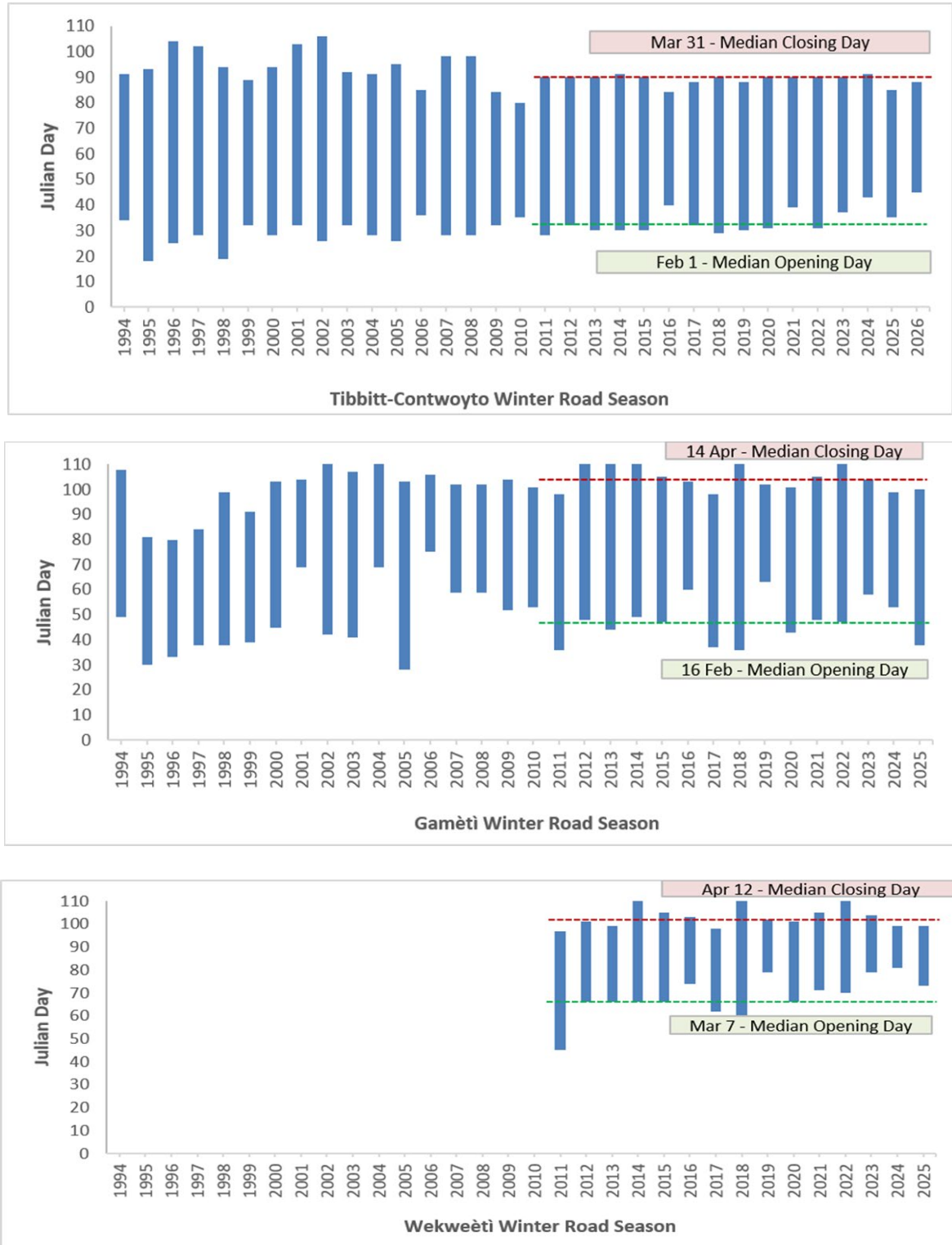
Figure 1-D. Opening and closing dates for the Tibbit to Contwoyto Winter Road (TCWR), Gamètì Winter Road, and Wekweètì Winter Road from 1994 to 2026. Data sources: GNWT Department of Infrastructure and TCWR Joint Venture Website ( jvtcwinterroad.ca ).
