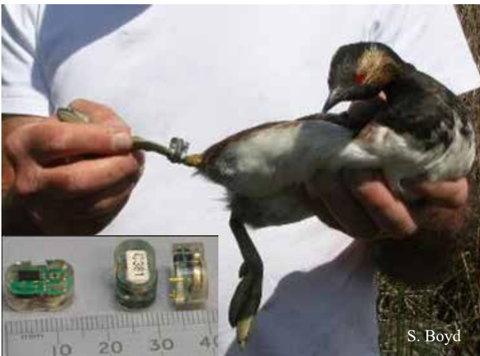
Figure 3. Geolocator attached to leg band on an Eared Grebe, a grebe that is slightly smaller than a Horned Grebe. Inset: geolocator with ruler to show size (14x8x6mm, weight:1g).
